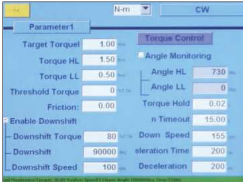
interface of tightening parameter setting
